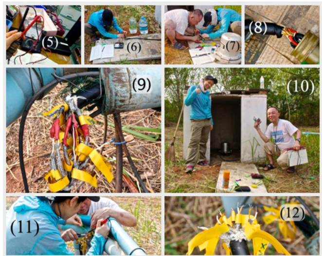
< Figure 2 : Testing and reconnecting the magnetometer's cable >
